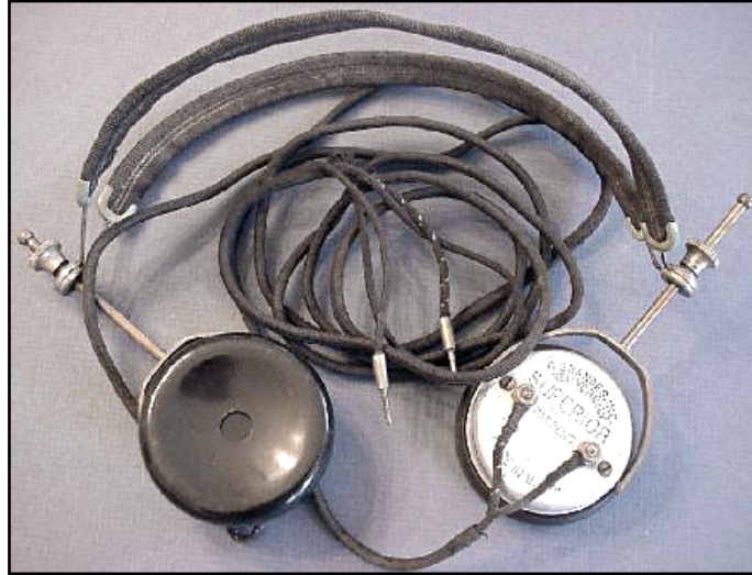
Fig. 1: First commercial headphone — Brandes Superior Matched Tone, circa 1919-21 (courtesy: Wikipedia Commons)
